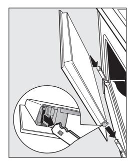
Hold the door securely at both sides and carefully fit it back onto the hinge guides. Make sure that the door goes back on straight.
